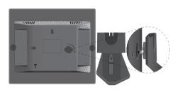
2. Rotate the foot stand counter-clockwise until it is secured to the digital photo frame.
